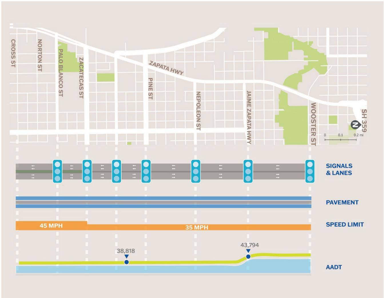
Figure 126 - Zapata Highway multimodal features
